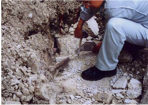
Photo.6 ㄱ ㄱ ㄱ Execution failure of movable joint part of EPS anchor
